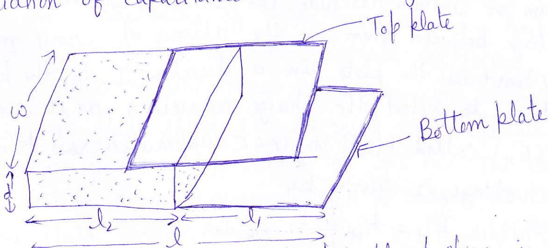
Fig. 3.17 Capacitive Transducer using the principle of change in dielectric constant for the measurement of displacement
