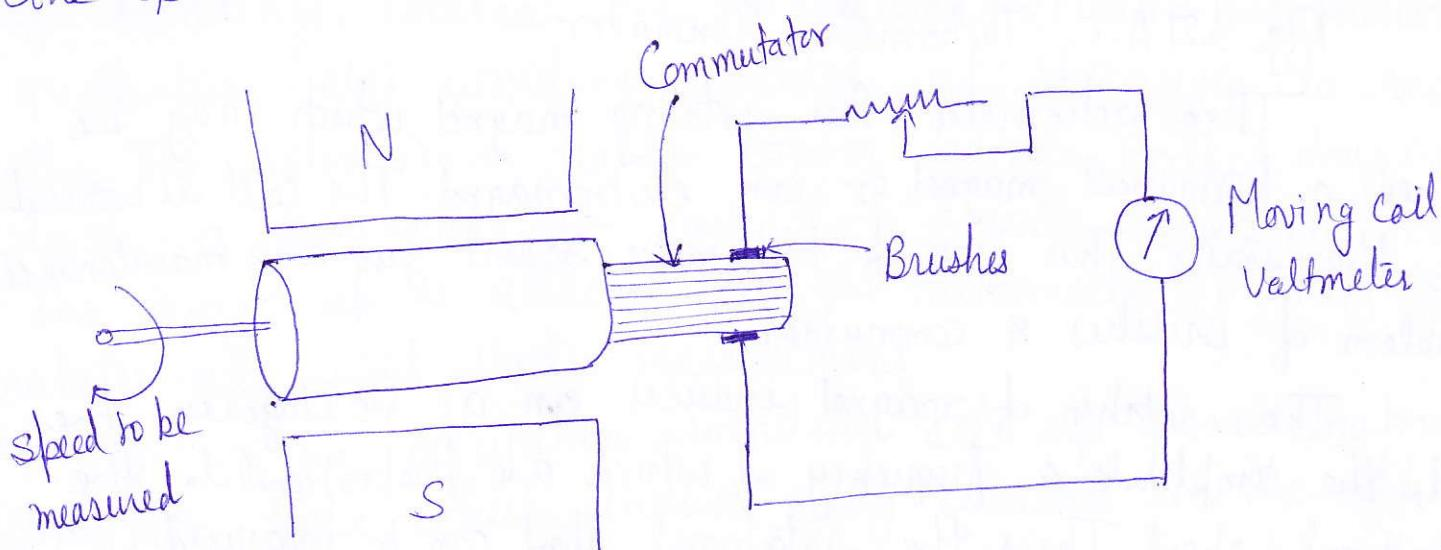
Fig. 3.26 D.C. Tachometer Generator
