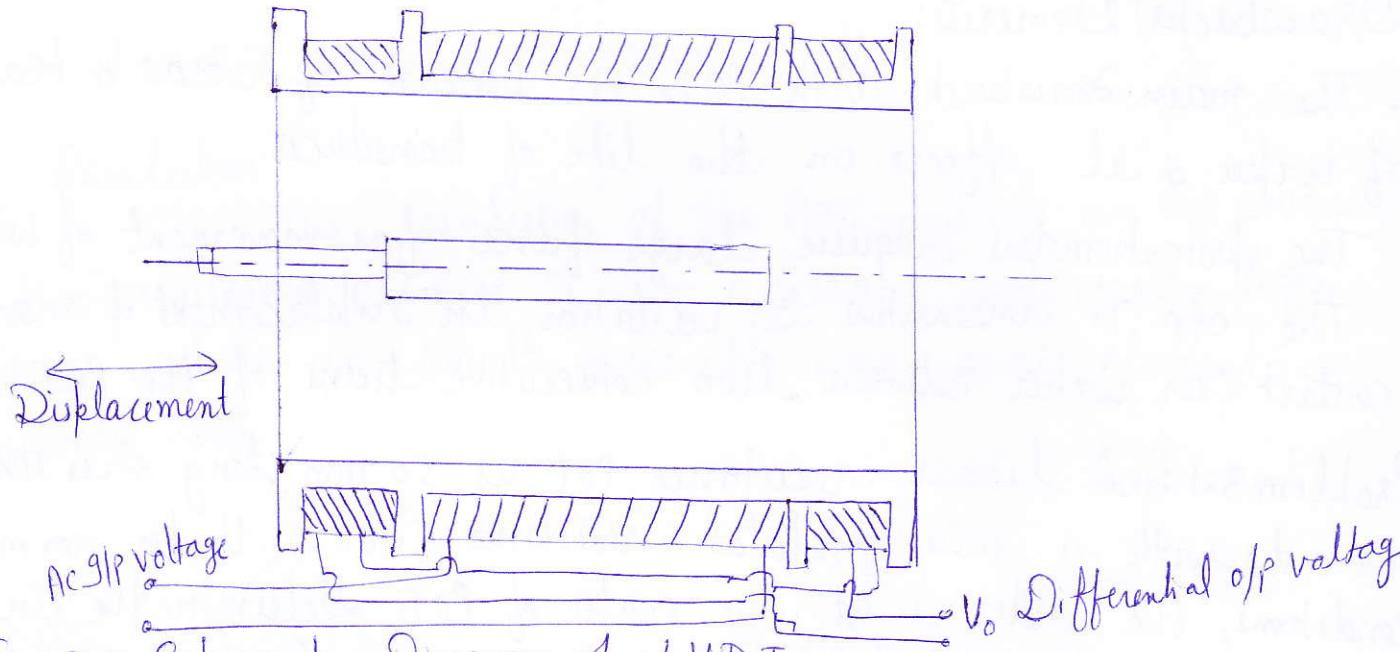
Fig. 3.9 Schematic Diagram of LVDT
