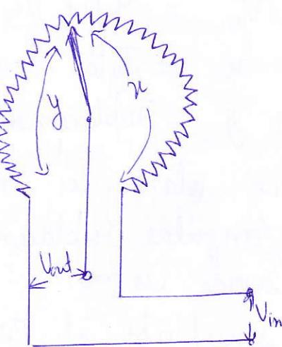
Fig. 3.2 Rotary Potentiometer
