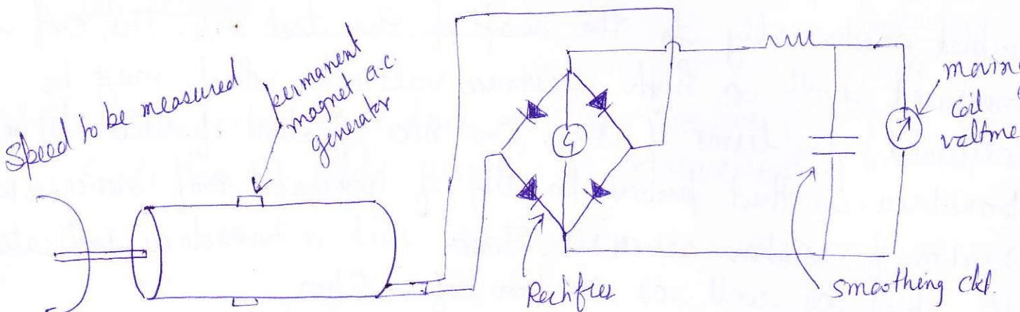
Fig. 3.27 A.C. Tachometer Generator
