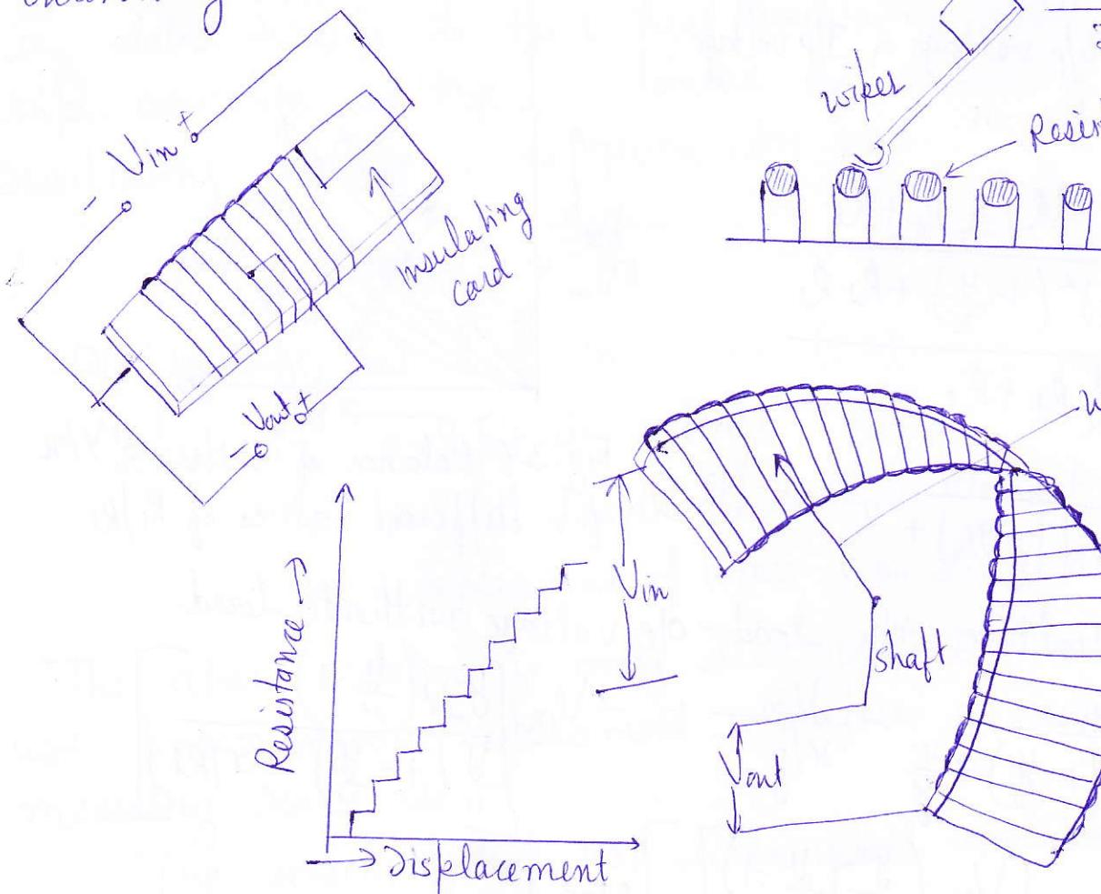
Fig. 3.8 Translatory & Rotational Motion of Potentiometer
