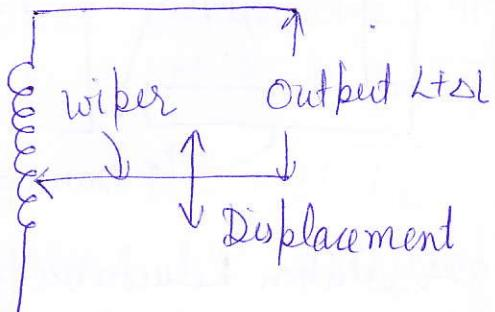
Fig. 3.19 Inductive Transducer for measurement of linear displacement
