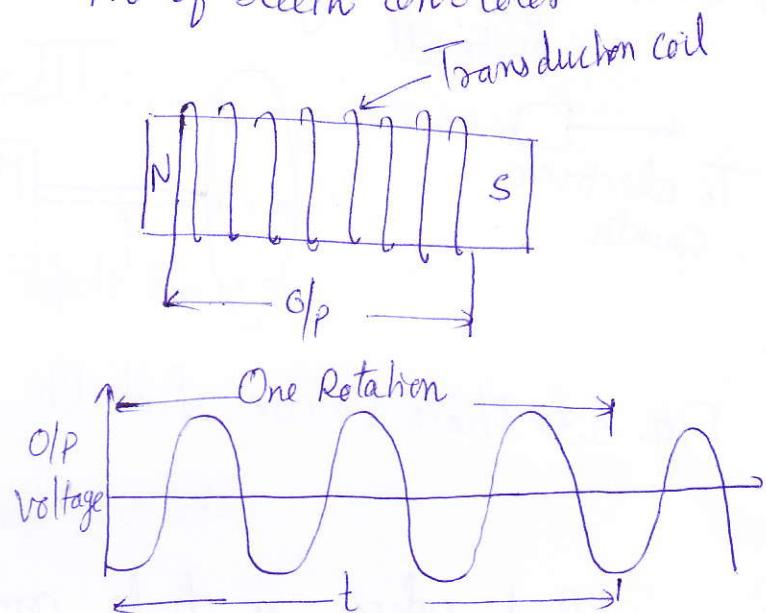
Fig. 3.29 Toothed Rotor Tachometer
