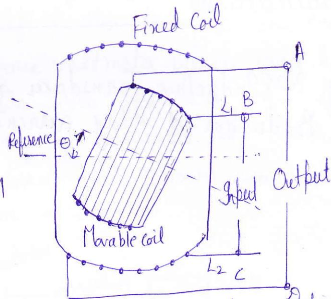
Fig. 3.34 Inductive Transducers working on principle of change in mutual inductance
