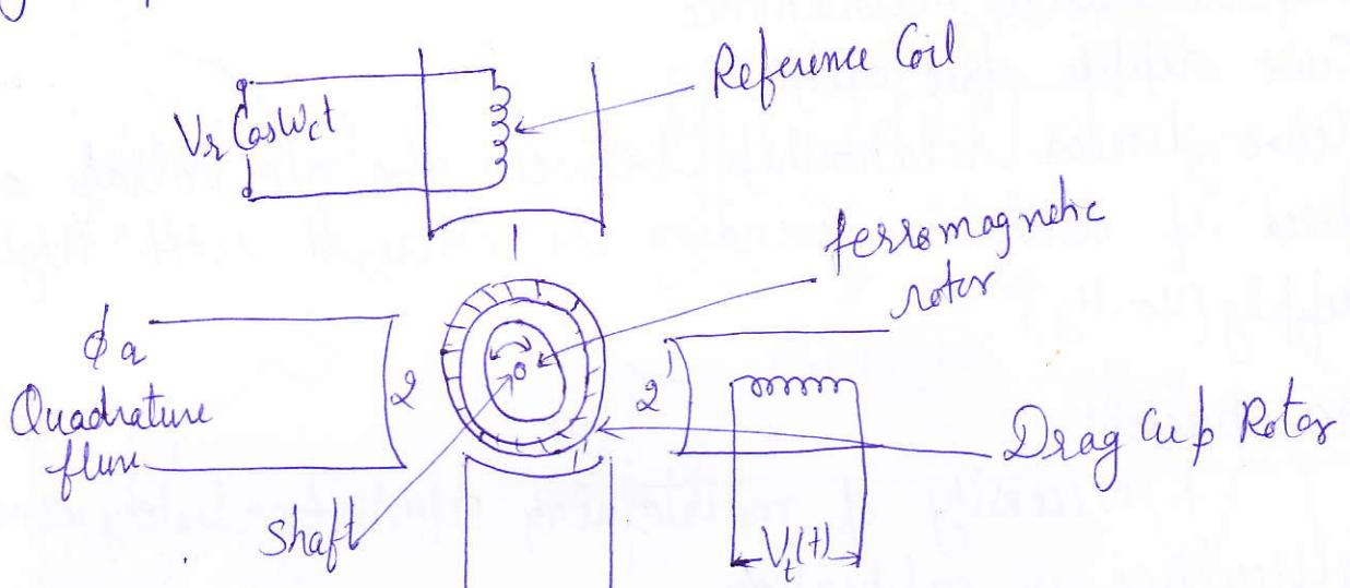
Fig. 3.28 Drag Cup Rotor A.C. Tachometer
