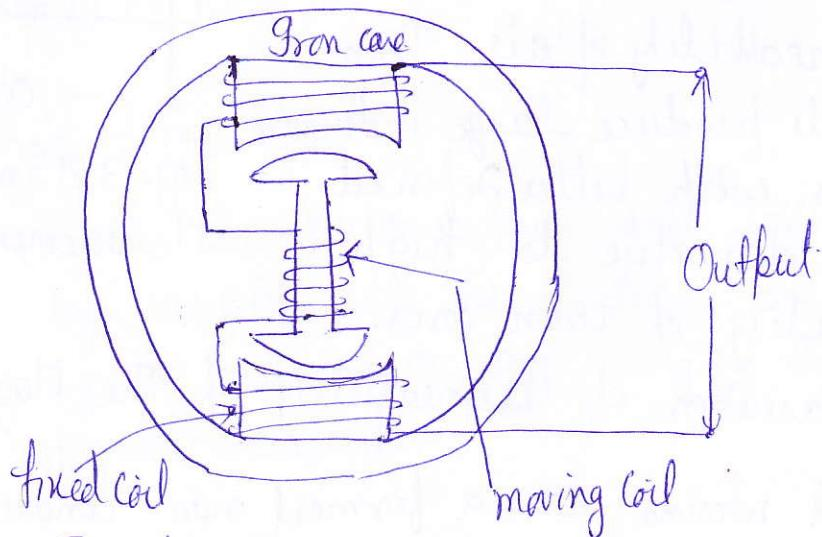
Fig 3.23 Inductive Transducer.
