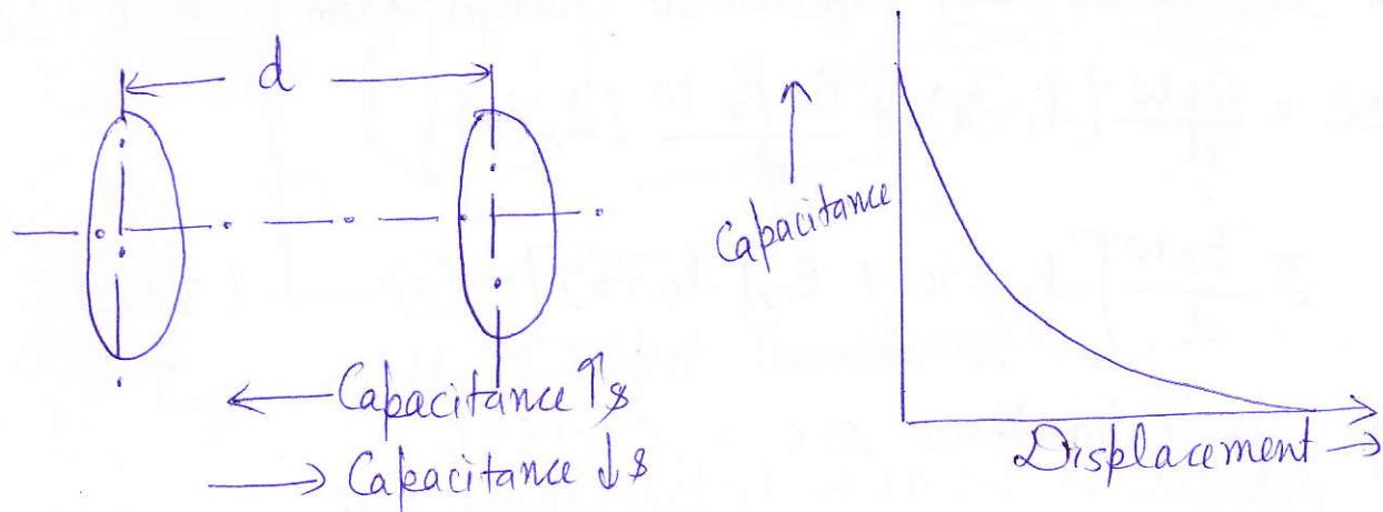
Fig. 3.16 Capacitive Transducer using the principle of change in displacement between the capacitor plates.
