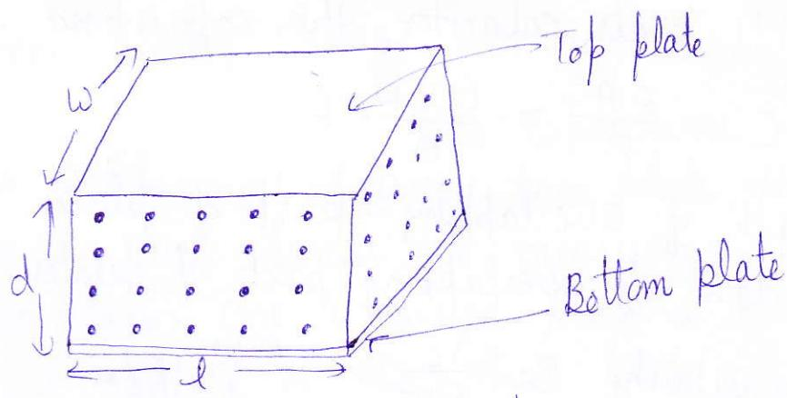
Fig. 3.13 Schematic diagram of Capacitive Transducers
