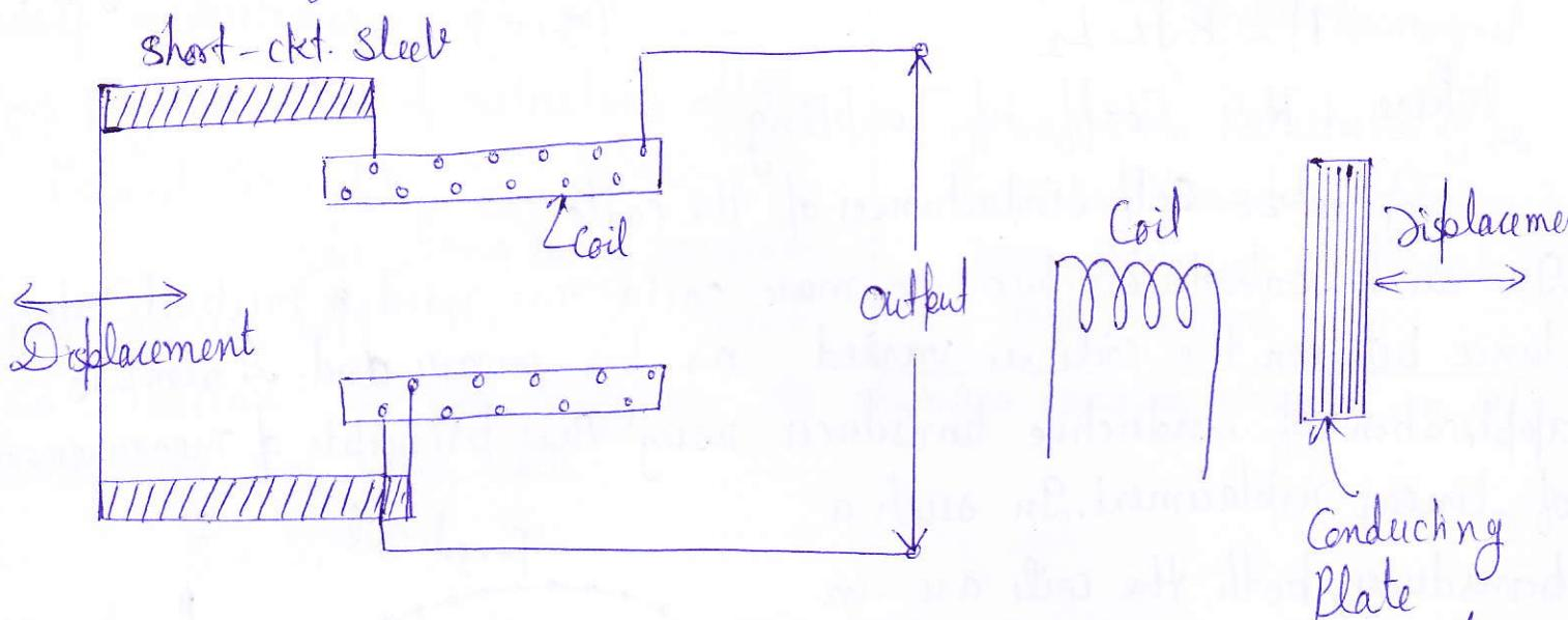
Fig. 3.25 Inductive Transducer working on the principle of Production of eddy currents for measurement of linear displacement
