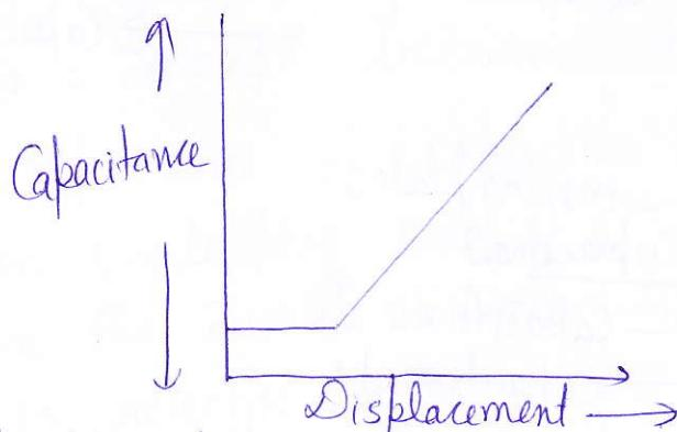
Fig.3.15 Capacitive Displacement curve for Capacitive Transducer.
