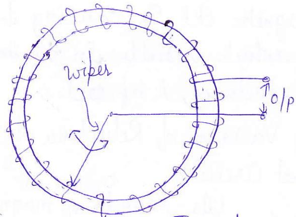
Fig. 3.20 Inductive Transducer for Measurement of angular displacement
