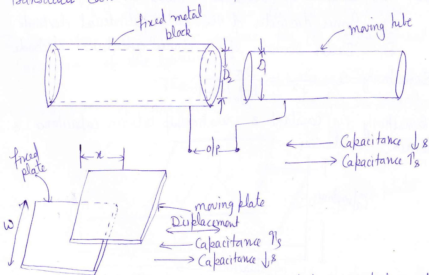
Fig. 3.14 Capacitive Transducer working on principle of change of capacitance with change of area.
