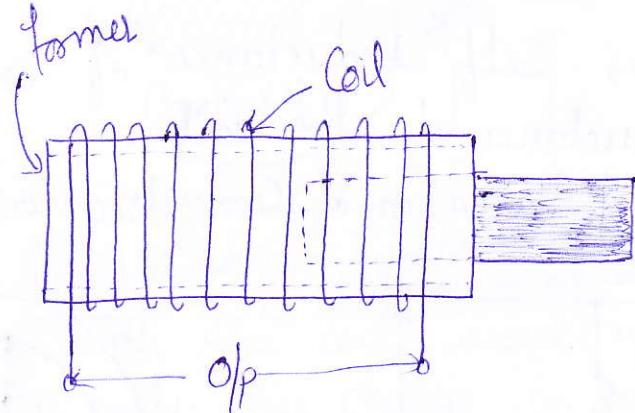
Fig. 3.21 Inductive Transducer for Measurement of Linear Displacement
