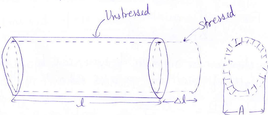
Fig. 3.12 Piezo Resistive strain Gauge
