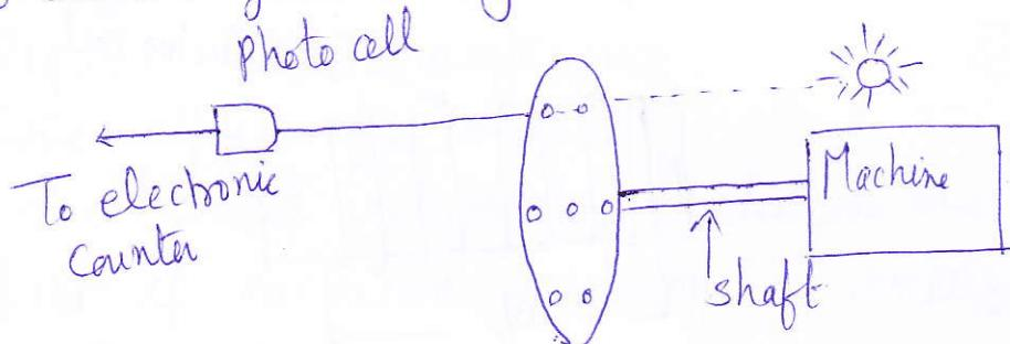
Fig. 3.30 Photo Electric Pick Up Tachometer
