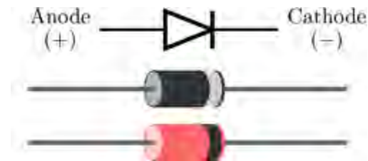
Figure 7: Typical diode packages in same alignment as diode symbol. Thin bar depicts the cathode.
