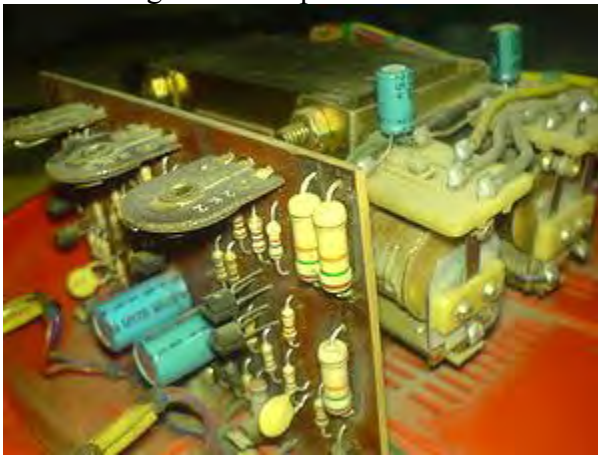
□ Interior of an old electromechanical voltage regulator.
